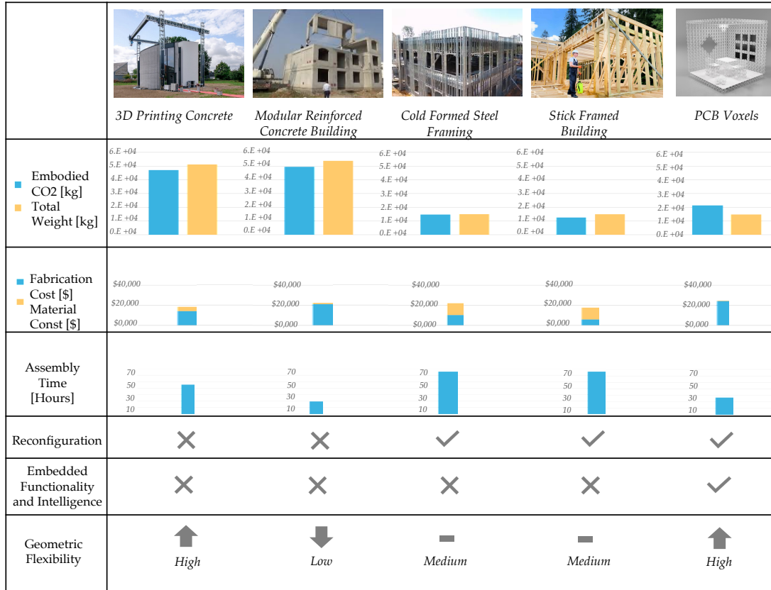
Figure 8.2: Large Scale Digital Fabrication Methods Comparison (data from [112]).
