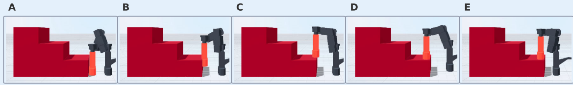
Figure 4.3: The locomotion catalog. (a) the seven families, in side view for the sagittal ones and top view for the lateral ones. Gray is the start stance and teal the end stance, while the red annotation gives each family's vertical vocabulary in voxels and the badge counts its actions. (b) two of them frame by frame in the simulator. Top strip, forward, the free foot arching over the planted foot to land half a voxel ahead (A–E). Bottom strip, climbUp2, the free foot swinging onto the step top and the body transferring up and over (B–E).
