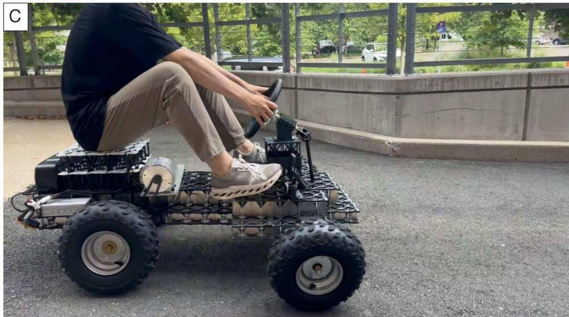
Figure 6-31: A) Kids mobility vehicle concept from Toyota. B) Coarsely voxelized version. C) Assembled main chassis under operation.
