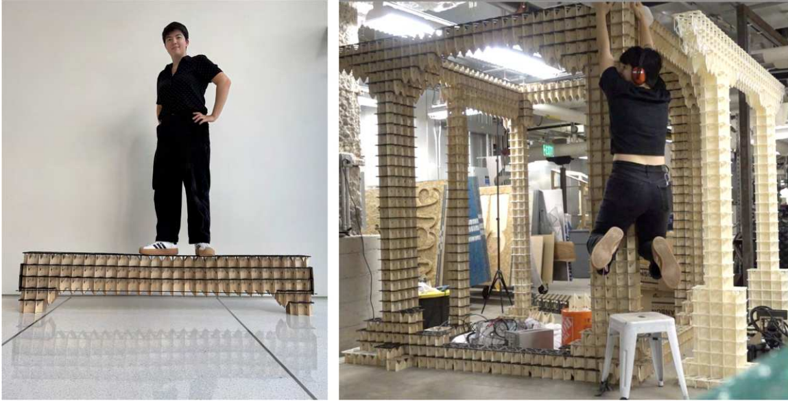
Figure 6-20: (Left) Post tensioned beam with human load. (Right) Testing the tiny house.
