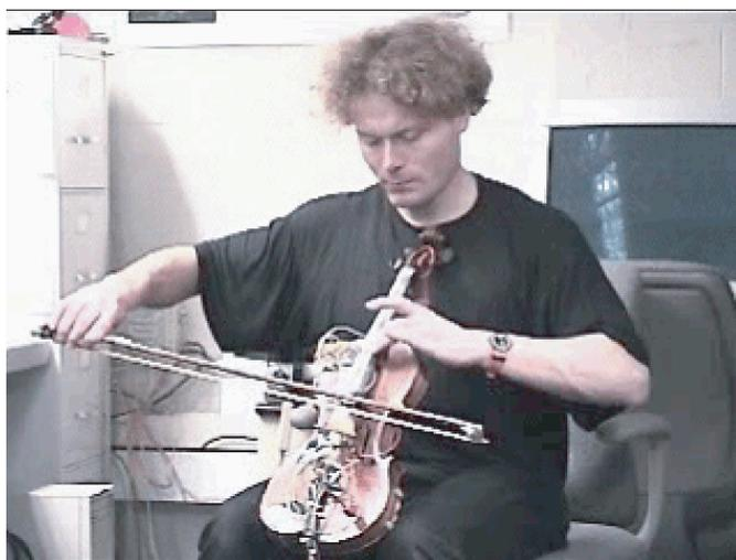
Figure 10-5: A one string digital violin (fall 1998). The strings are muted. The instrument functions as a sensor input device for the single-string model, ranging over two octaves. A sound clip is available from [WEB].
