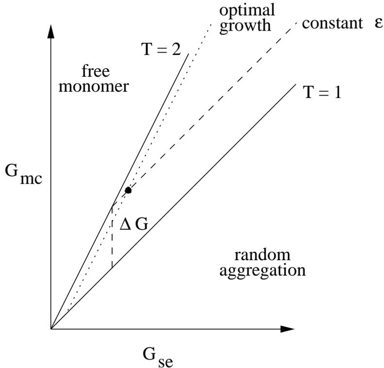
Figure 10: Analysis of the phase diagram for 2D self-assembly. Lines mark the melting transition  $\mathcal{T} = 2$ , the precipitation boundary  $\mathcal{T} = 1$ , a line of constant error rate  $G_{mc} = G_{se} + \Delta G$ , and the line on which optimal growth rates occur  $G_{mc} = 2G_{se} - \ln 2$ .
